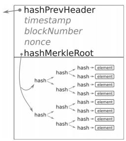
The blocks of actual blockchain data structures include, in the block header, some optional, but useful, information such as the timestamp when the block was created, the sequence number of the block in the chain, and possibly a nonce, a random number chosen to fulfill certain properties and generated as part of the block creation process.
