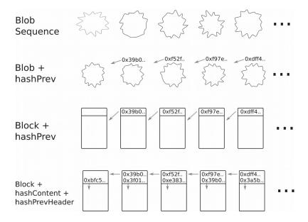
At its most fundamental, the blockchain data structure consists of an ordered sequence of chunks of data, a sequence of binary blobs.
