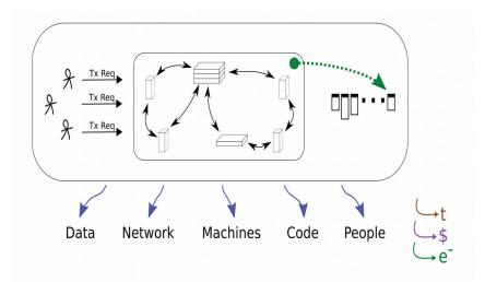
A blockchain project, structurally, consists of data flowing through the computation, of a network enabling the exchange of messages, of machines to process and store information, of software code to perform those operations, and of the people involved in all phases of the project. Maintaining all of these requires time, money, and electricity.
