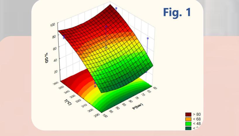
Fig. 1 represents the 3D plot and 2D contour plot for the percentage of green diesel as a function of pressure and temperature. Results suggested that green diesel yield increseed when increasing temperature, while the effect of hydrogen pressure appears moderate.
