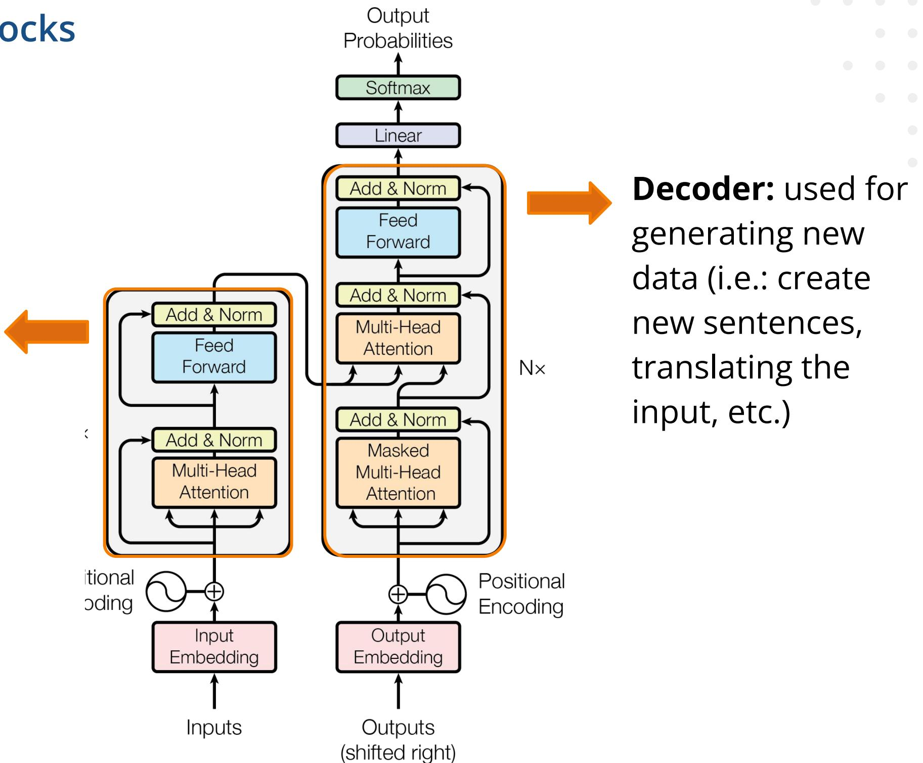
**Decoder:** used for generating new data (i.e.: create new sentences, translating the input, etc.)
