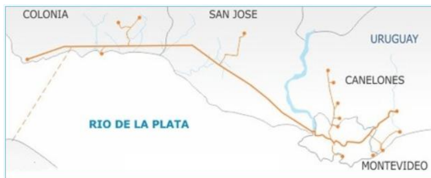
Figure 11. Gasoducto Cruz del Sur S.A. (GCDS) runs from Punta Lara in Argentina to Montevideo and its surrounding areas in Uruguay, traversing the departments of Colonia, San José, Canelones, and Montevideo (Gasoducto Cruz Del Sur, 2025)
