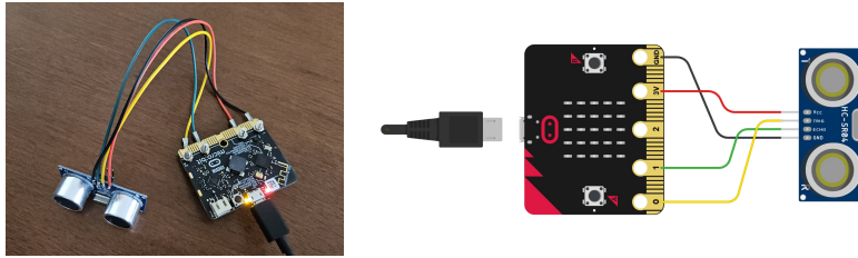
Figure 1: Connection setup used in MissionMotion , showing the micro:bit board connected to an ultrasonic distance sensor and interfaced with a laptop for real-time motion acquisition. When using micro:bit, the HC-SR04P ultrasonic sensor must be employed instead of the HC-SR04, as it is compatible with the 3.3 V operating voltage of the micro:bit.
